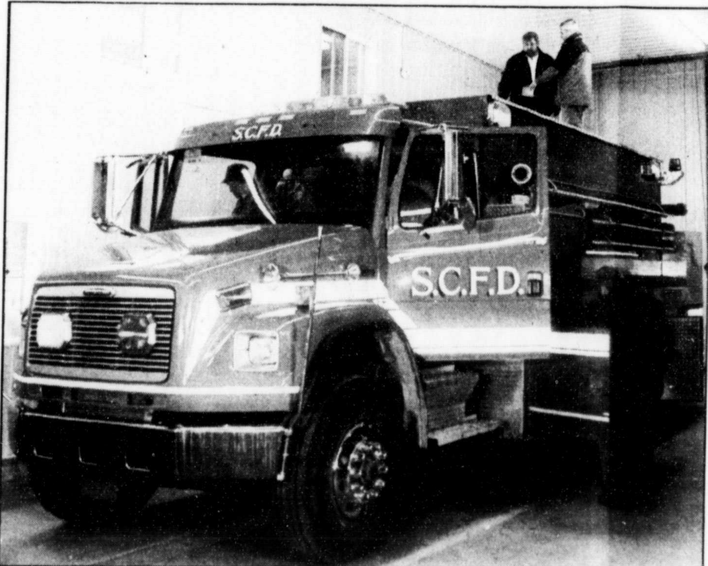
THE TANKER THAT CAN: Firefighters can now haul and pump more water to the scene of a fire anywhere in Clarendon or Shawville. The Shawville-Clarendon Fire Department took delivery of a new 3,000 gallon tanker March 12. The 2002 FreightLiner was built to department specifications, touting a 350 h.p. power plant. It has three outlets, three inlets and can pump up to 600 gallons a minute at 25 psi. Pictured above is Clarendon Mayor Jack Lang, left, with Al Ruzen of Advance Engineered Products, Concord, Ont builders of the tanker, mulling over the new machine.
