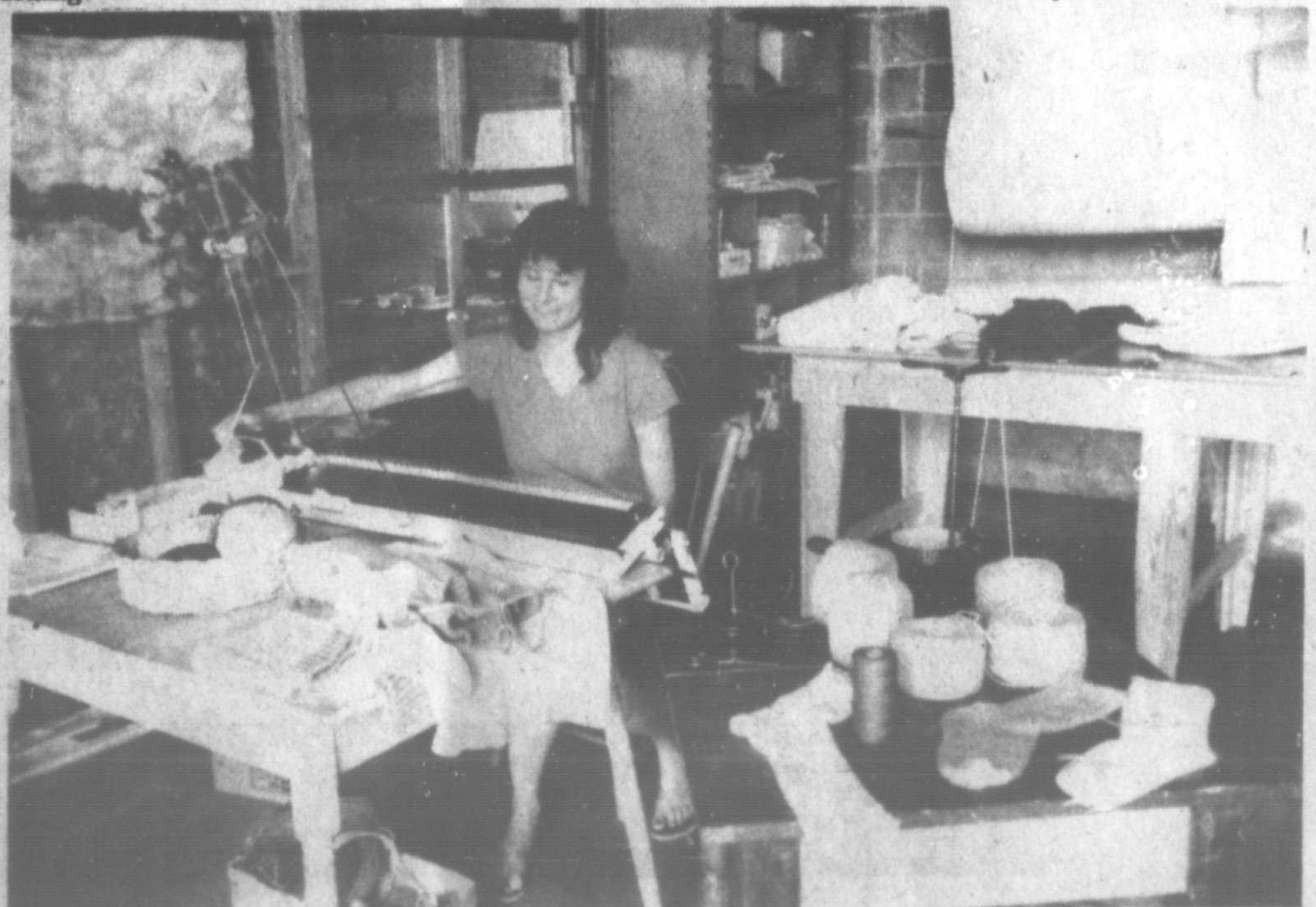
Marilee has become expert at the automatic knitting machine. Behind her are rolls of felt made from the wool of Pontiac sheep. The felt is used to make boot liners, slippers, for horse blankets and other items, all handmade at the Wool Works.
